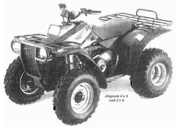
Magnum's 425 4-stroke and 34mm constant velocity carb have a big appetite for work. Automatic transmission, single-lever, all-wheel hydraulic disk brakes, too.
